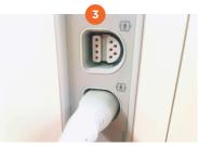
Connect the ANI MOC-9 module to one of three MOC-9 ports on Root
