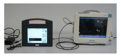
Figure 2: Example for connecting to the Philips MP50 monitor
